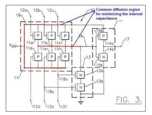
• Internal capacitance of the logic gate also is a major roadblock in increasing its speed. The internal capacitance of the gate also typically limits the number of logic inputs which can be handled by a single gate
